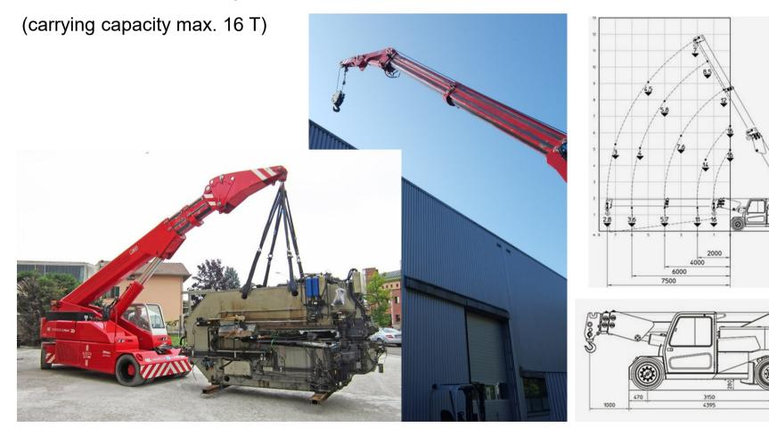
**Capabilities cabin-controlled portable crane**
